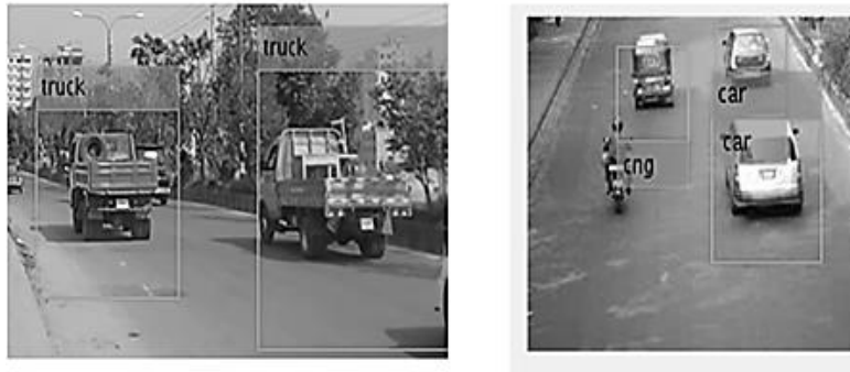
Fig. 12: Detected vehicles are classified in a video (Scene 1)
