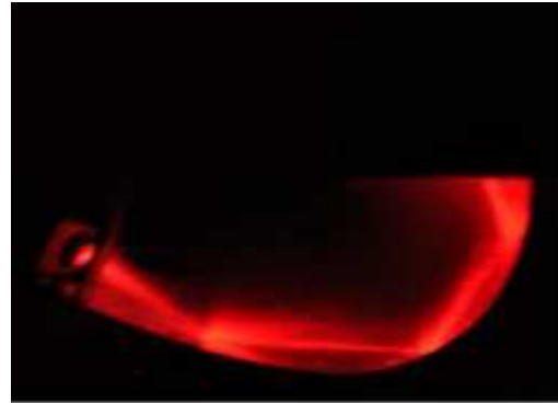
Fig. 9: (f) Test-5, Laser (Three reflections) on lower parabola and circular reflector of CTAH
