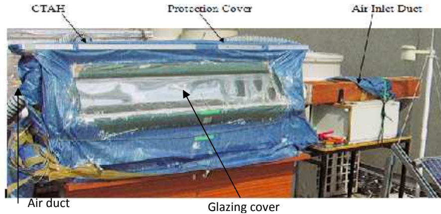
Fig. 3: Outdoor experimental setup with CTAH and long inlet duct
