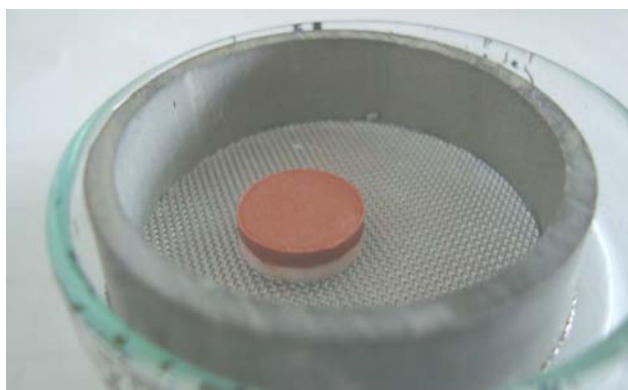
Figure 1. Device used to measure water uptake and swelling of the bilayered buccal tablets
