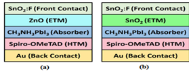
Fig. 3. (a) Model cell 1: \text{TiO}_2 is replaced by ZnO (b) Model cell 2: \text{TiO}_2 is replaced by \text{SnO}_2 .
